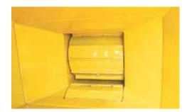
TWIN HORIZONTAL FEED ROLLERS. A 23 x 35.5 cm infeed opening fed by oversized horizontal offset feed rollers helps allow material at maximum capacity to be efficiently fed to the chipper.
