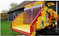
**SMARTFEED.** The SmartFeed system monitors engine rpm and automatically stops and reverses the feed rollers to maximize production. This system also senses feed roller jams and manipulates the material automatically to reduce the need for manual control bar use.
