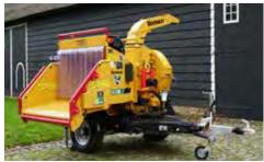
**CONVENIENT TURN-TABLE.** Allows the chipper infeed to be rotated into seven positions to face the material for ease of feeding and convenience when working along the roadside. An optional height-adjustable surge brake is available for the BC230.
