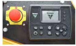
ECOIDLE™ ENGINE CONTROL SYSTEM. When the Ecoldle system is selected by the operator, the engine speed automatically lowers to a preset rpm after one minute or five minutes of inactivity to help reduce fuel consumption when not chipping material. This idling can help reduce
