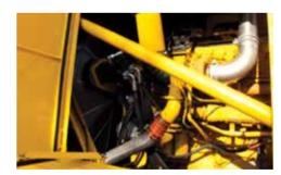
**ENGINE POWER.** A CAT C27 Tier 4i (Stage IIIB), Twin Turbo engine provides 950 hp (708 kW) of power to meet your jobsite demands.
