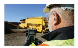
FULL-FUNCTION REMOTE. The ability to adjust the working trommel screen from the loader is made possible by the standard full-function remote control. The remote allows you to adjust screening functions, raise and lower conveyors, pause the hopper, reverse the engine fan and more.
