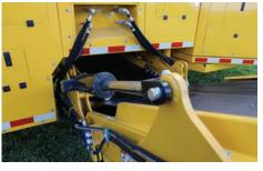
JOBSITE FLEXIBILITY. The auxiliary hydraulic system grants the TR6450 trommel screen the ability to run the third fraction conveyor or other attachments.
