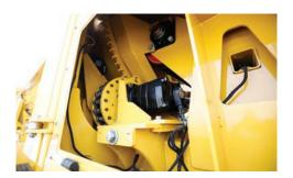
**DRUM DRIVE.** The hydraulic-driven chain drive system provides positive drum drive and also allows the drum to lift off of the cog for service and maintenance. The drum drive is monitored so the hopper belt will stop when the drum is reaching capacity, in order to prevent over feeding.
