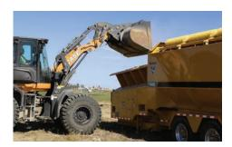
**LOW HOPPER HEIGHT.** With a hopper height of 9.5 ft (2.9 m), the operator can load material without having to build a ramp to the machine, decreasing loading cycle times.
