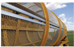
TENSIONED SCREEN DRUM. Tensioning the screens allows for maximum strength with a fine wire gauge, optimizing production through improved open area. In high moisture applications, the use of stainless steel screens can be very useful.
