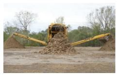
3-PRODUCT PRODUCTION. The optional third product conveyor allows the single drum TR6450 trommel screen, to produce three unique products in one pass.
