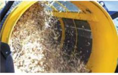
**HIGH PRODUCTION.** The tensioned screens around the drum add rigidity, allowing use of smaller-gauge wire — helping increase production capacity and enable processing of wetter material.
