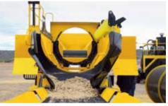
**MINIMAL CLEANUP.** Flashing and sheeting fit tightly against the drum to help reduce spillage.
