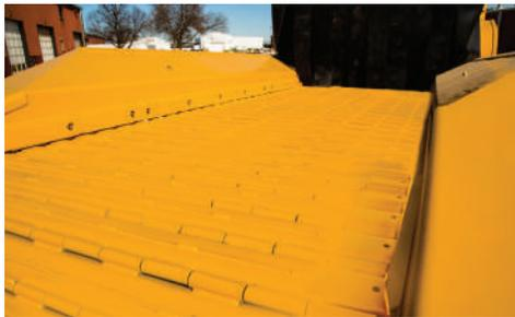
**CONVENIENT FEEDING.** The HG6800Tx features low side walls to aid in feeding whole trees and other larger material with less restriction, reducing the number of user interactions with the material.
