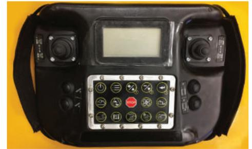
**CONVENIENT CONTROL.** The transceiver remote is equipped with a fault log, machine control menu, and the ability to supply the user with machine-operating information to monitor the machine's health.
