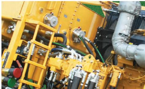
**DURABLE HYDRAULIC CIRCUIT.** Independent hydraulic circuits are an important factor in limiting contamination to the affected circuit and its respective components.
