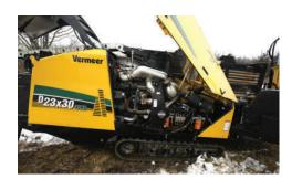
PREMIUM POWER. A 100 hp (75 kW) Deutz TCD3.6L4 engine provides power to help drive the D23x30pr S3 to its peak performance, while a thrust/pullback of 24,000 lb (106.8 kN) combines with rotational torque of 3000 ft-lb (4067.5 Nm) to help get the drill into tough ground.
