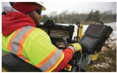
**ROCK QUIETLY.** Following the reliable S3 sound badge, the D23x30pr S3 has an operator ear noise level of 83 dB(A) to help with operator comfort, crew communication and create a guiet working environment to reduce disturbance to neighborhoods and other populated urban areas.
