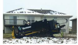
WORTH ITS WEIGHT. Weighing in at 16,500 lb (7484.3 kg), the D23x30pr S3 is the lightest rock drill in its class. The lightweight design helps keep your jobsite intact by decreasing potential disturbance to sidewalks, neighborhoods and landscapes.
