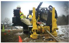
COMPACT CONTROL. A width of 55.5" (141 cm) makes the D23x30pr S3 drill 24.5" (62.2 cm) narrower than its closest competitor, offering efficient maneuverability of the machine into compact urban areas or busy neighborhoods, and convenient transportation on a trailer with other equipment.
